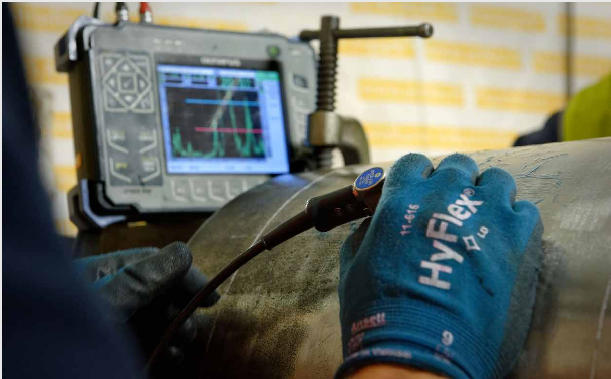
ULTRASONIC EXAMINATION OF WELDS
