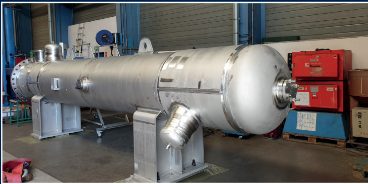
◀ EASU EXCHANGER, N2 NUCLEAR PRESSURE EQUIPMENT, DESIGNED ACCORDING TO THE RCC-M CODE © ONET TECHNOLOGIES
